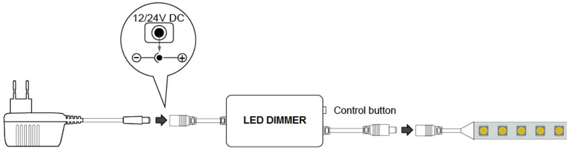
Application Circuit 2: CW+WW(power input by DC male plug 2.1/5.5, led output by 4 pin\*2.54 connector: V+ CW NC WW)
